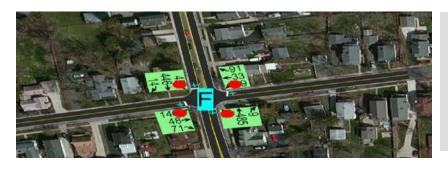
The through traffic filling up the local streets is responsible for the higher delays at this Intersection. Heavy left and right turns.
