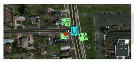
The Intersection delay is 3.1 sec but the delay on East Bound lane is pretty high 79 sec.
