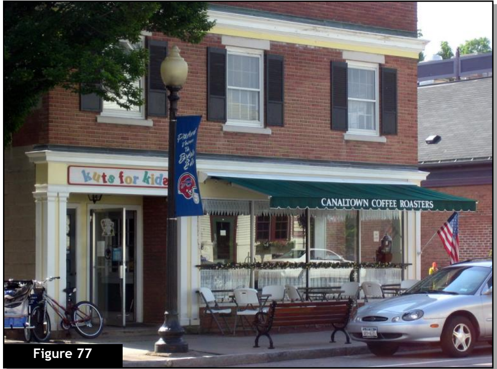
Figure 77 Awnings are a high quality design element that define the purpose and volume of outdoor spaces. They also add visual variety and distinction to building façade components [§ 112-16G(4)(h)]. The building in Figure 77 also displays a significant amount of transparency and the successful use of a cornice to differentiate the 1st floor from upper stories.
